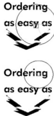
Figure 7. Experimental example where connections between CCs are shown. The region R(CC_i) of character “y” contain the centroid of character “n” but the two characters are not connected because the centroid of character “y” is out of the region R(CC_j) of character “n.”
