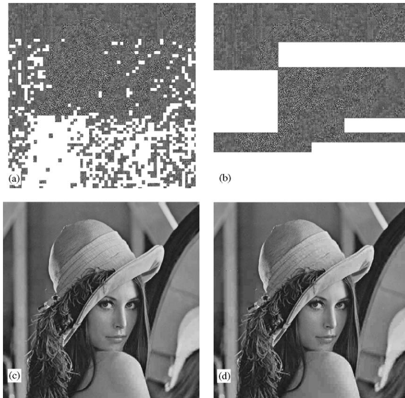
Fig. 8. The effect of a congested network on the reconstructed image: (a) reconstructed MSL-coded residual image, (b) reconstructed tiled & JPEG-coded residual image, (c) final reconstructed MSL-coded image and, (d) final reconstructed tiled & JPEG-coded image.
